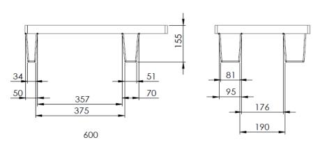
\*All load capacity data is only valid in case of evenly distributed load. For all indicated dimension tolerances of +/- 3 mm apply.
