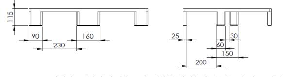
\*All load capacity data is only valid in case of evenly distributed load. For all indicated dimension tolerances of +/- 3 mm apply.
