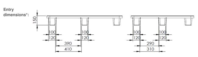
\*All load capacity data is only valid in case of evenly distributed load. For all indicated dimension tolerances of +/- 3 mm apply.
