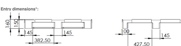
\*All load capacity data is only valid in case of evenly distributed load. For all indicated dimension tolerances of +/- 3 mm apply.
