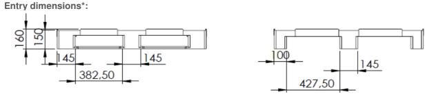
\*All load capacity data is only valid in case of evenly distributed load. For all indicated dimension tolerances of +/- 3 mm apply.
